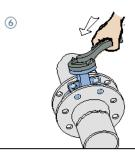
After welding seams cooled down, slide in the butterfly valve. Make sure there is enough space for the valve and the disc is slightly open.
